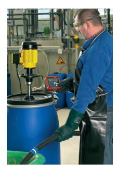
Lutz flow meters of series TSB can be used for most different applications. They are suitable for the measurement of thin-bodied up to medium-viscous and inflammable liquids. Due to a battery-powered option, series TSB can be also ideally used for a mobile operation, independent from a mains system.
