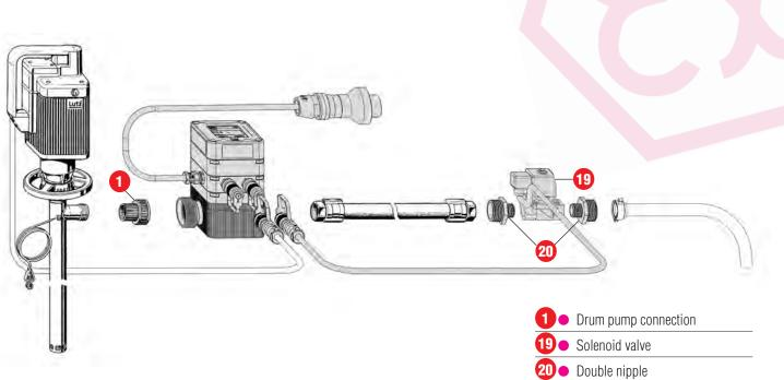
... with thread connection to a drum and container pump (Ex)
